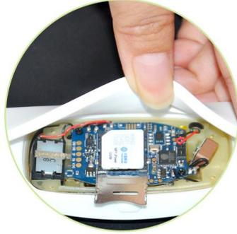
2. Open the SIM card slot, insert micro SIM card, then close the slot cover
