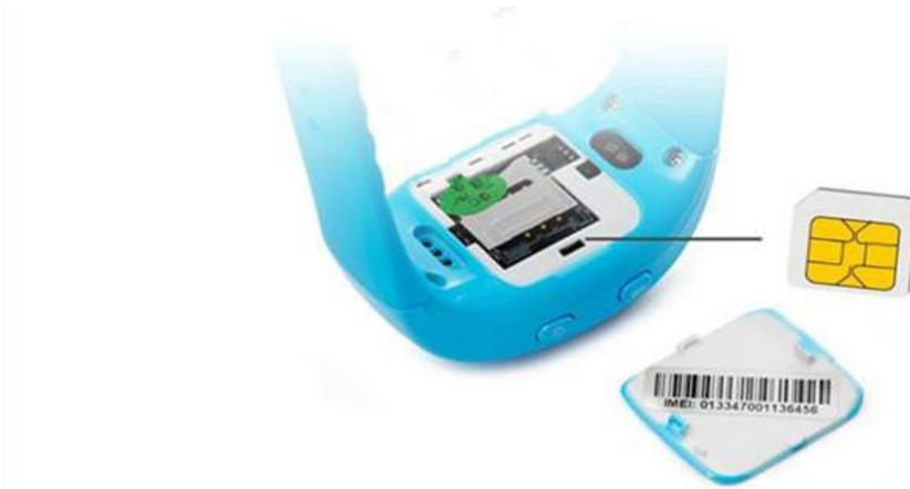
2. Press the power button to start the device after the SIM card and back shell is installed correctly.
